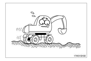
When operating in water or when crossing shallow, check the bed soil condition and depth and flow speed of water, then proceed taking care that water is not above axle center.
